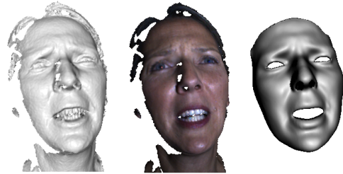
Figure 1: From left to right, the image shows the 3D reconstruction of a person's face, the corresponding texture mapped on it, and the spatio-temporal consistent representation of the face surface.
